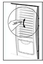
Airflow direction adjustment Up-and-Down.
